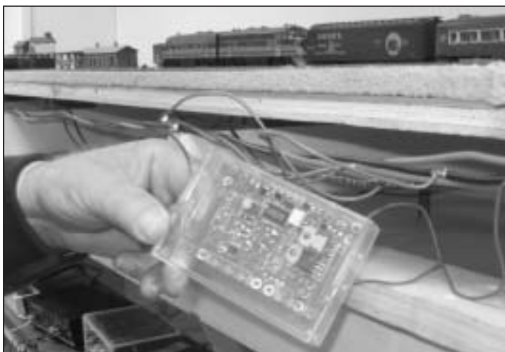
Franklin uses empty audio cassette cases as protective enclosures for his high-speed DCC circuit breakers. Free protection for delicate parts!
