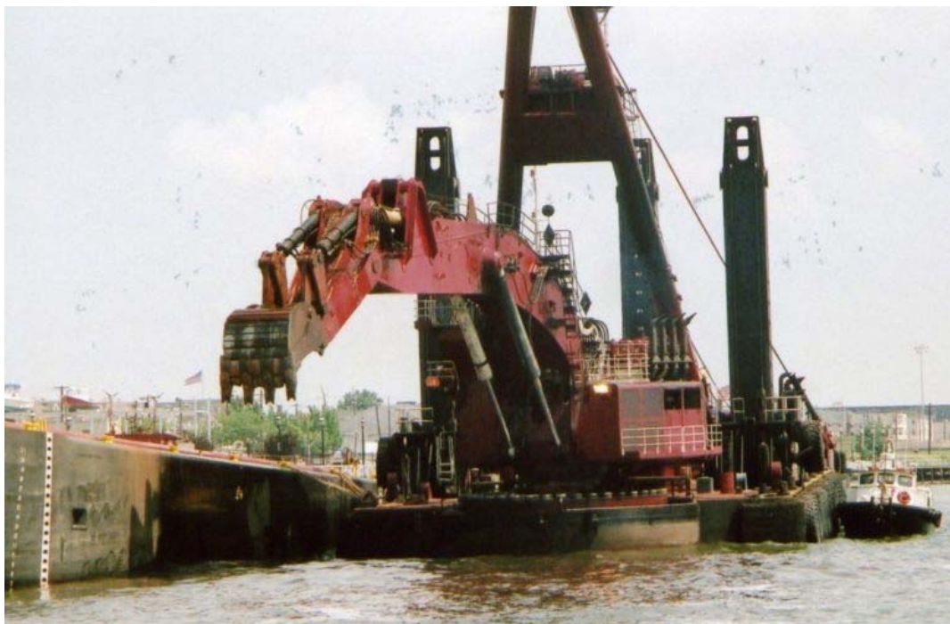
There's more than one way to dig a hole! - Great Lakes Dredge and Docks floating dredge at the Elizabeth River outlet into Arthur Kill
